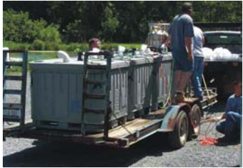
Side view of the fish transport truck and trailer with four insulated seafood totes used during the study. Each tote was equipped with aerators, air vents, gas flow meters and gas diffusers.
