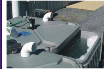
Top view of an insulated seafood tote used to transport live Arctic char ( Salvelinus alpinus ) during the study. Totes were equipped with aerators and filled with 850-900 L of 13°C spring water.
