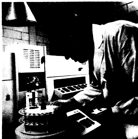
Figure 2. Atomic absorption is a relatively new analytical technique that facilitates the determination of plant nutrients and makes leaf analysis more useful because of the broader and more accurate analysis.
